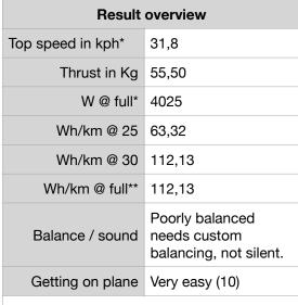
\*Top speed and power are taken from peak moments so results might differ from full power consumption \*\*Note, measurement of full speed consumption in based on short trips, which may result in less precise data compared to the 25/30kph tests that cover a greater distance.
