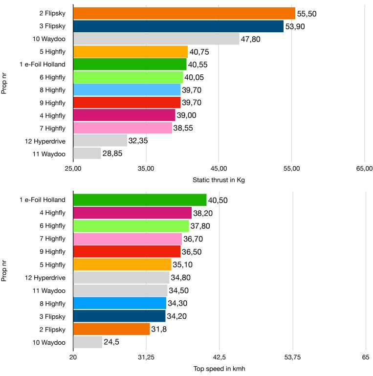
It is important to note that the results of the thrust test may vary due to several factors. These factors include the weather conditions, electrical connections, battery health,
