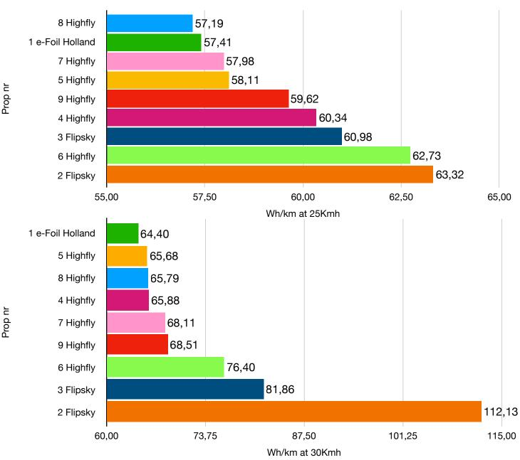
It is important to note that the results of the propeller efficiency test may vary due to several factors. These factors include the rider's weight, weather conditions, electrical connections, battery health, and riding technique. Each of these elements can have an impact on the overall performance and efficiency of the E-Foil system. Therefore, while the test provides valuable insights, it is essential to consider these variables and their potential influence when interpreting the results.
